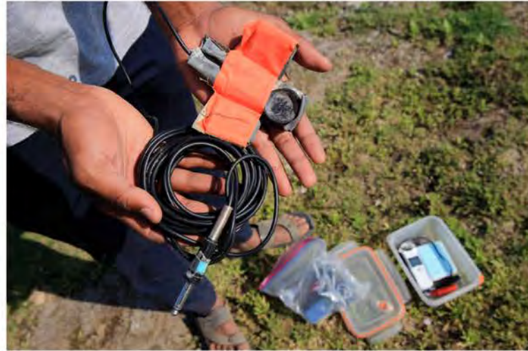
Photo 18. The hydrophone (circular disc adjacent to red tape), weighted with lead, is submerged in shallow water, and attached by cable to a digital recorder. Typically, a dual array is installed each monitoring period, for hours of observation recorded. In some settings, these arrays are left for 24-48 hrs so that remote continuous recordings can be made near breeding / nesting sites. This arrangement allows the GEP team to detect specific individuals.
