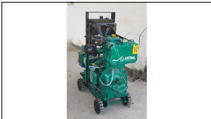
Fig. 113 Consistent and reliable power is required at both upstream and downstream bases, due to often irregular mainline power, especially during monsoon. Astral funding has provided a 5KVA genset for each base that will allow 24 hr power service with an inverter, for recharge and to provide backup service.
